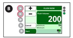
B. Press the + and – buttons to input the desired flush volume.
