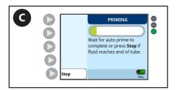
C. Kangaroo OMNI™ Enteral Feeding Pump will show a progress bar indicating the automatic prime is in process. Wait for the priming to complete.
