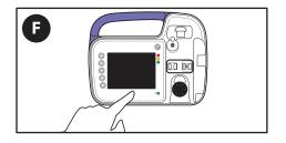
F. If alarm continues after replacing Kangaroo OMNI™ Feeding Set, press **Power Off** to stop operation and use a different Kangaroo OMNI™ Enteral Feeding Pump.
