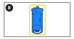
B. **Check** the tubing inside the cassette to ensure that it is free from lint or other debris.
