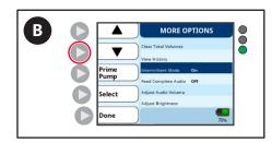
B. Press the down arrow button until Intermittent Mode is highlighted.
