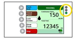
Kangaroo OMNI™ Enteral Feeding Pump status LED Indicator lights on the upper right of the pump screen provide a quick visual indication of Kangaroo OMNI™ Enteral Feeding Pump status.
