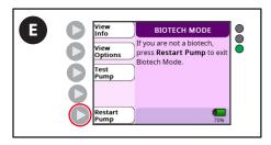
E. Press the **Restart Pump** button to save the settings and exit Biotech mode.
