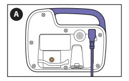
A. Plug the power adapter into the power adapter port located on the back of Kangaroo OMNI™ Enteral Feeding Pump.
