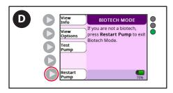
D. Press the **Restart Pump** button to save the settings and exit Biotech mode.
