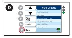
D. Press the **Done** button to return to the Ready to Feed screen. The **Adjust Feed** button will now appear and Feed settings can be adjusted.
