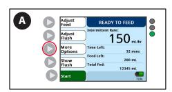
A. Press the **More Options** button on the Ready to Feed or Set Loaded screen.
