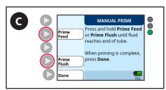
C. Press and hold the **Prime Feed** or **Prime Flush** button until the solution just begins to exit the distal connector.
