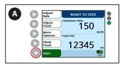
A. Press the **Start** button to begin feeding. **Note:** Start button will only appear when all feed or all flush parameters have been entered.
