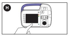
H. If alarm continues after replacing Kangaroo OMNI™ Feeding Set, press **Power Off** to stop operation and use a different Kangaroo OMNI™ Enteral Feeding Pump.
