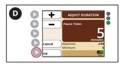
D. Press the **OK** button to confirm the desired pause time. The Timed Paused screen will show a time countdown until the pause duration is complete.
