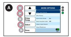
A. In the More Options screen, use the arrow keys to select **Adjust Brightness**, and press the **Select** button.
