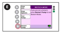
E. Press **Restart Pump** button to save the settings and exit Biotech mode.
