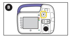
B. Check the valve actuator for blockages and confirm the valve actuator is correctly oriented.
