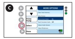
C. Press the **Select** button. "On" or "Off" will be displayed to indicate the present Intermittent Mode state.
