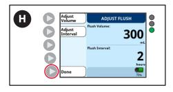
H. Press the **Done** button to confirm the time interval and return to the **Ready to Feed** screen.
