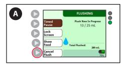
A. Press the **Cancel Flush** button to stop a Flush Now that is in progress and return to feeding.
