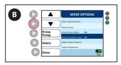
B. Press the down arrow button until Feed Complete Audio is highlighted.
