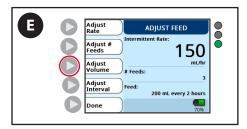
E. Press the **Adjust Volume** button to set the Feed volume.
