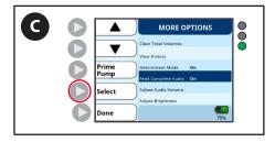
C. Press the **Select** button to toggle the audio between "On" and "Off".
