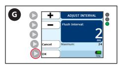
G. Press the **OK** button to confirm the time interval and return to the **Adjust Flush** screen.
