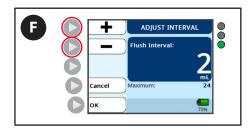
F. Press the + and – buttons to input the desired time interval.
