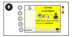
B. Press **Continue** and prime the pump to prepare for next flush. Disconnect patient from tubing before priming.
