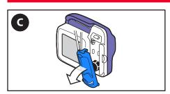
C. If alarm continues, **turn off pump** and **Remove** the cassette from Kangaroo OMNI™ Enteral Feeding Pump.
