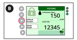
B. To disable the Lock Screen and reactivate buttons, press and hold the **Unlock Screen** button for 5 seconds.
