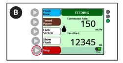
B. To change the rate or feed setting once feeding has started, press the **Stop** button.
