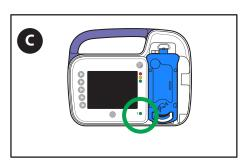
C. Confirm the green Power Indicator Light is on to ensure Kangaroo OMNI™ Enteral Feeding Pump is receiving power.
