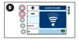
B. Press the + and – buttons to input the desired volume.
