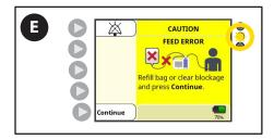
E. **Confirm** the audible alarm, color display, and colored LEDs all properly indicate a Feed Error condition.
