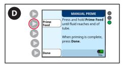
D. Press and hold the **Prime Feed** button until the feeding solution just begins to exit the distal connector.
