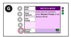
G. Press the **Restart Pump** button to save the settings and exit Biotech mode.
