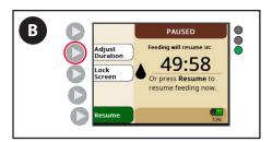
B. To adjust pause duration from 5 minutes, press the **Adjust Duration** button.
