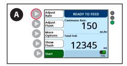
A. Press the **Adjust Rate** button to set the continuous feeding rate.
