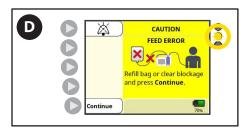
D. Upon priming, Kangaroo OMNI™ Enteral Feeding Pump will detect a Feed Error condition and alarm.
