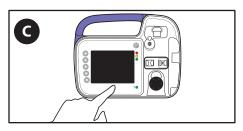
C. If alarm continues after replacing Kangaroo OMNI™ Feeding Set, press Power Off to stop operation and use a different Kangaroo OMNI™ Enteral Feeding Pump.
