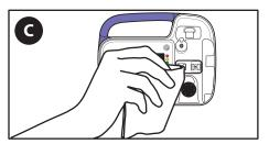
C. **Clean and dry** the Kangaroo OMNI™ Enteral Feeding Pump occlusion sensor region. For excessive cleaning needs, avoid use of sharp objects during the cleaning process. Use of a soft bristle brush for example may be used.
