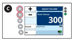
C. Press the + and – buttons to input the desired flush volume.
