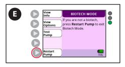
E. Press **Restart Pump** button to exit Biotech mode and return to normal operating mode.
